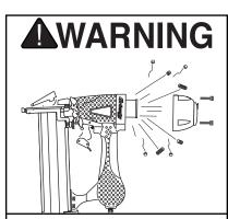
Exceeding the maximum permissible operating pressure may cause the nailer to explode, blowing metal fragments in all directions. To protect yourself from serious personal injury, DO NOT allow your air compressor to exceed the recommended pressure when connected to the nailer!
